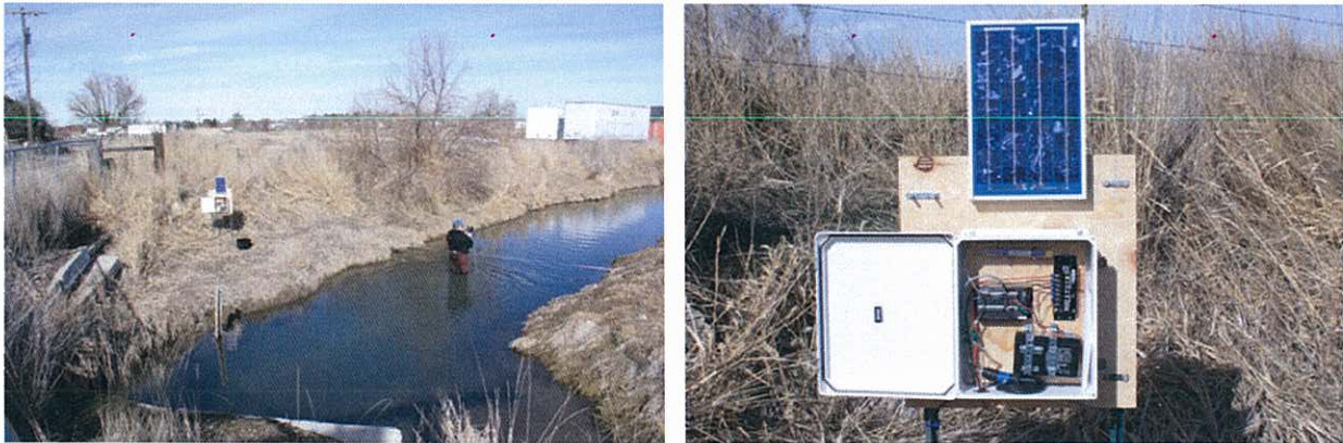
Figure 5 – Deployment of the DFM system at the Hartley Drain. In the left hand picture the DFM enclosure and power supply can be seen mounted on the far side of the Drain, the permanent staff gage is located in the Drain just in front of the DFM system, the sensor is located in the squash pipe just visible on the left hand side of the frame, and Department Hydrologist Dan Nelson is seen current metering the Drain in the right side of the frame. The right hand picture is a close up of the enclosure, data logger, and power supply.
